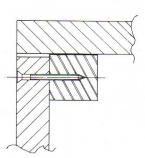
Versions of the reinforced butt joints shown above may be employed. The reinforcing battens should be 1" x 1" (25 mm x 25 mm) planed softwood. It is important that all surfaces of the joint are liberally coated with a suitable woodworking adhesive, to ensure that joints are both strong and airtight. Screws should be No. 8 or No. 10 countersunk and should be spaced no more than 6" (15 cm) apart. Screw lengths will be determined by the exact thickness of timber employed.
